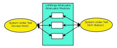
The LANforge attenuator sits between two RF systems, often a WiFi AP on one side and WiFi Station on the other. The attenuator and WiFi stations are connected by shielded SMA-Male cables. Adjust the attenuation as desired using either the attenuator knobs or use software to adjust the values over the USB-Serial connection.
