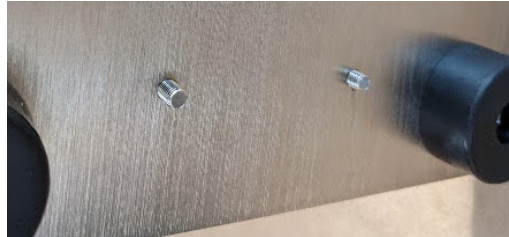
3. Add nuts to all four rods on bottom side of plate. Hand tighten.
