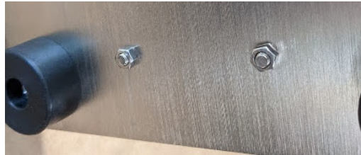
3. Add nuts to all four rods on bottom side of plate. Hand tighten.
