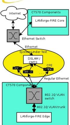
The CT570 configuration is an affordable way to use LANforge to generate network traffic on a large number of physical interfaces. LANforge uses its ability to support 802.1Q VLANs and an affordable 802.1Q VLAN switch to provide traffic generation on 24 or more physical 10/100 Ethernet interfaces
